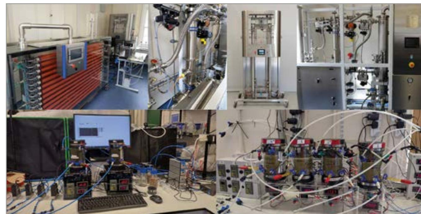
Figure 18. Examples of bespoke reactor designs developed for laboratory and pilot operations, some allowing up to 10 bar pressure operation.
